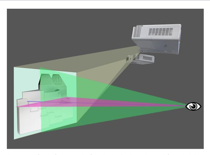
This test model features flat and curved surfaces, detail in the 7thSense logo, and a face with a highly detailed mesh, in front. Whilst the projectors are pitched down, the design eyepoint (red and green axis planes) is horizontal. Here is how each virtual projector in DeltaGUI will see the canvas (in this case a 3D object), and note that they may see surfaces the viewer is not designed to see, or even for which there is no media coverage:
